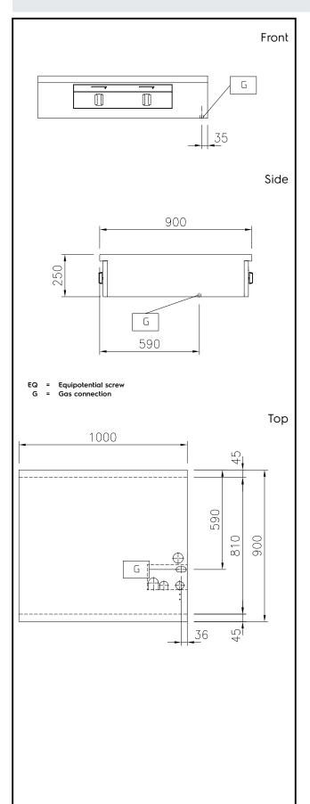
Gas Gas Power: 40 kW Gas Type Option: Gas Inlet: 1/2" **Key Information:** External dimensions, Width: 1000 mm 900 mm External dimensions, Depth: External dimensions, Height: 250 mm Net weight: 82 kg Configuration: Two-Side Operated;Top ISO 9001; ISO 14001 - ISO 9001; ISO 14001 kW Front Burners Power: **Back Burners Power:** 10 - 10 kW **Back Burners Dimension -**Ø 70 Ø 70
